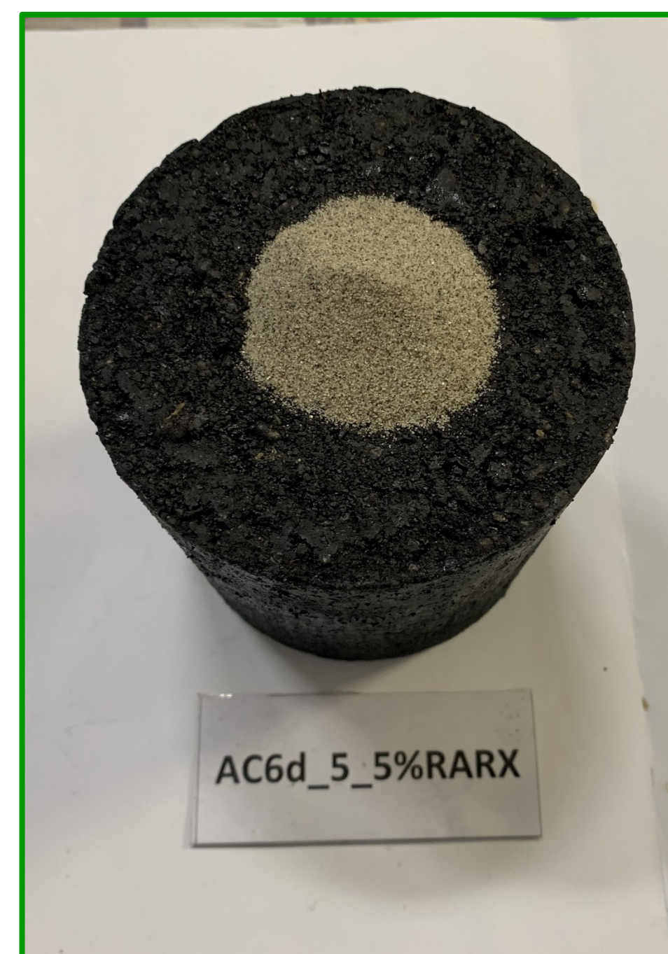
Sand Patch Test
