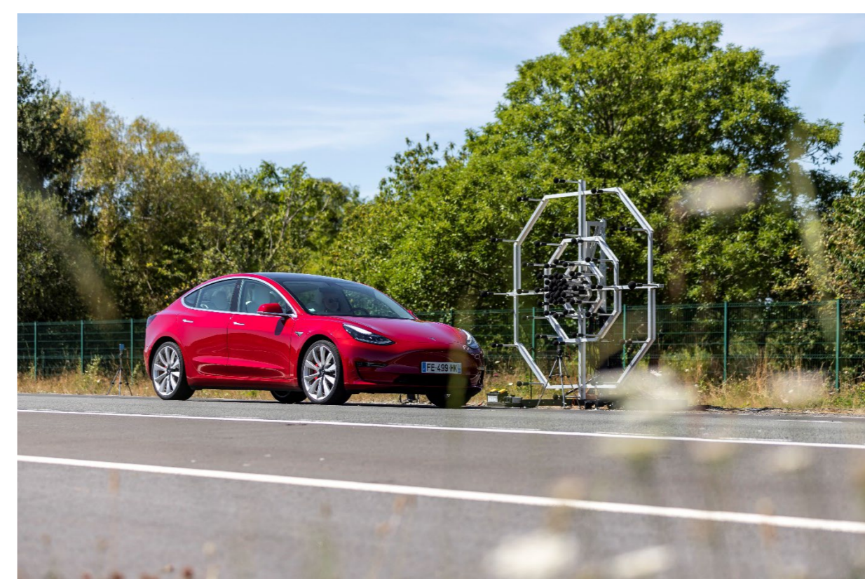
Microphone array measurement at pass-by of a BMW i3s (left) and TESLA Model 3 (right)
