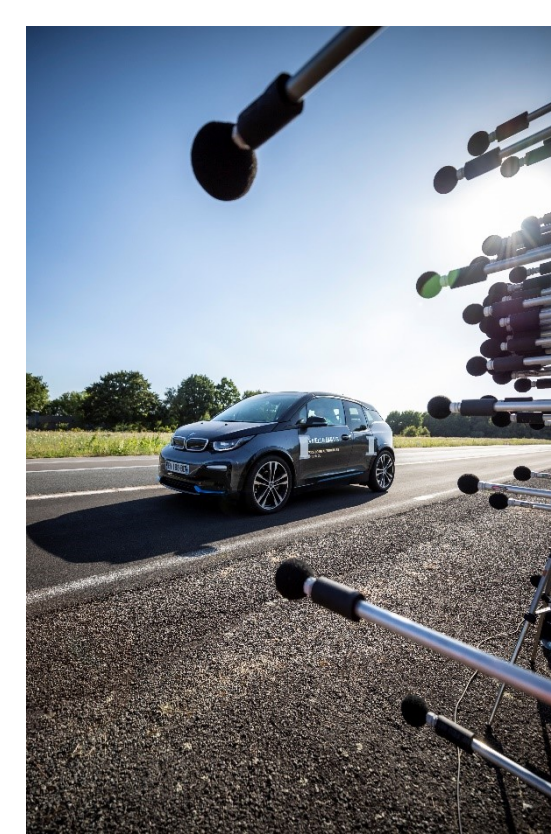
Microphone array measurement at pass-by of a BMW i3s (left) and TESLA Model 3 (right)
