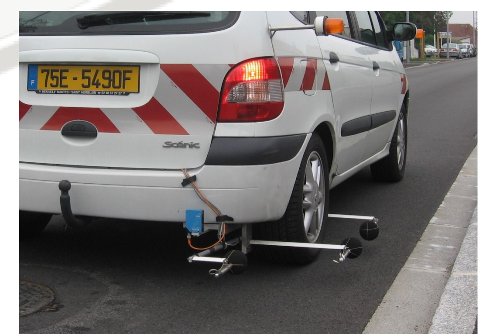
On-board continuous noise measurement system (CPX)
