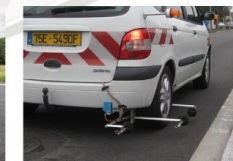
On-board continuous noise measurement system (CPX)
