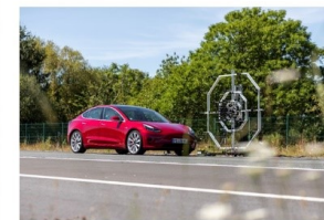
Microphone array measurement at pass-by of a BMW 13s (left) and TESLA Model 3 (right)
