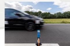
Infrared cell for speed measurement during vehicle noise measurement at pass-by
