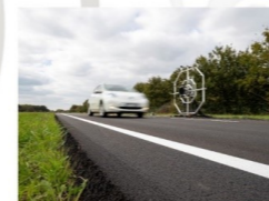
Microphone array measurement at pass-by of the Nissan LEAF on the prototype road
