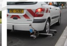
On-board continuous noise measurement system (CPX)
