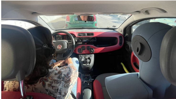
Figure 4 - Binaural recordings inside the vehicle
