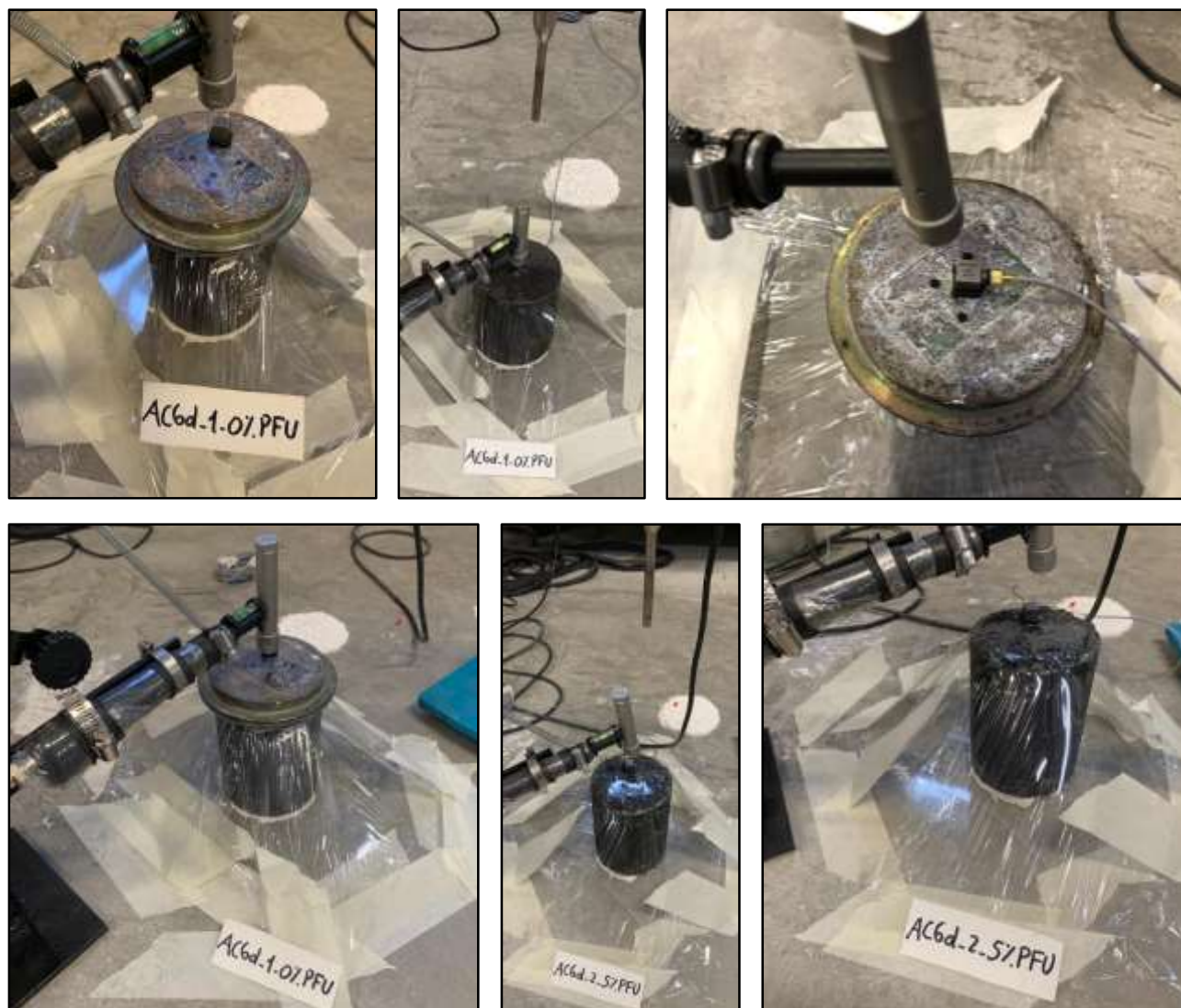
Figure 13. Set up used to derive the mechanical impedance in laboratory
